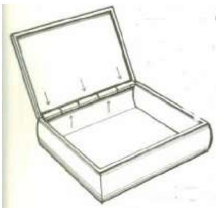
*The above diagram illustrates how the knuckles of the integral hidden-hinge snuff box are formed alternately from the lid and back of the box*
